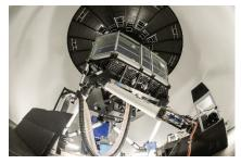
The Large Motion Simulator in the SOSc with a moving bridge of  $4 \times 5 m$  on a hexapod.
